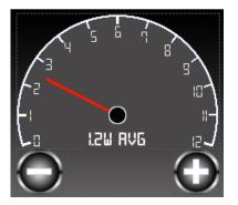
The power dial shows the preset power and the average power emission based on the pulse type.
