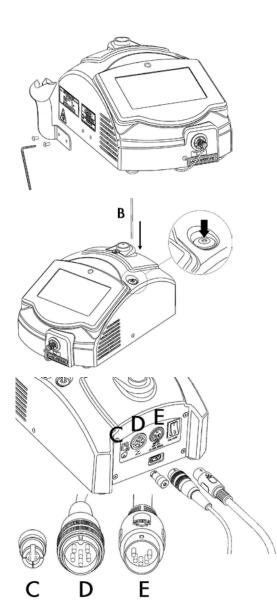
**1.** Place the laser body on a flat steady surface. Attach the handpiece holder to the laser body using the screws and key supplied.
