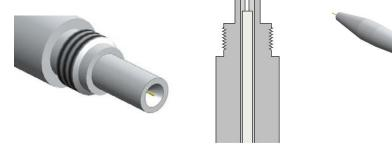
2. Insert the fibre into the handpiece until it reaches the top. The fibre <u>must not exit the</u> <u>border of the adaptor</u>, as shown in the diagram. If necessary, adjust the output length of the fibre by unscrewing the bottom cap
