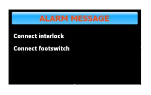
**3.** The system will verify that the footswitch and interlock are in place. If they are not the following error warning will appear.
