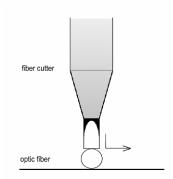
Step 1: place the cutter perpendicular to the fibre
