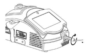
**2.** Plug the fibre connector into the socket on the laser body and turn the connector clockwise until it comes to a complete stop.
