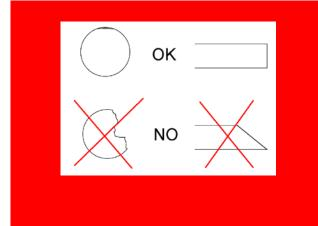
WARNING: the aiming beam is a good means of verifying the integrity of the system . If the beam spot is missing from the distal extremity of the transmission and if the intensity is reduced or seems diffused, this can indicate that the transmission system has deteriorated or is not working properly.
