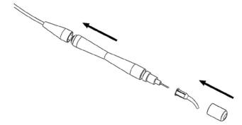
3. If necessary, adjust the output length of the fibre by unscrewing the bottom cap.
